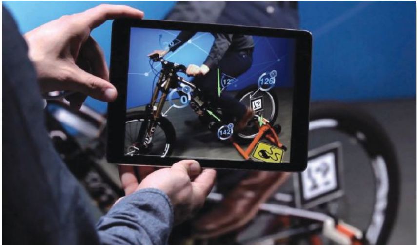
At LiveWorx 2015, PTC demonstrated the concept of a digital twin using an iPad augmented reality app. The speed and turn angles shown on display are real-time data transmitted from sensors. Image courtesy of PTC.
