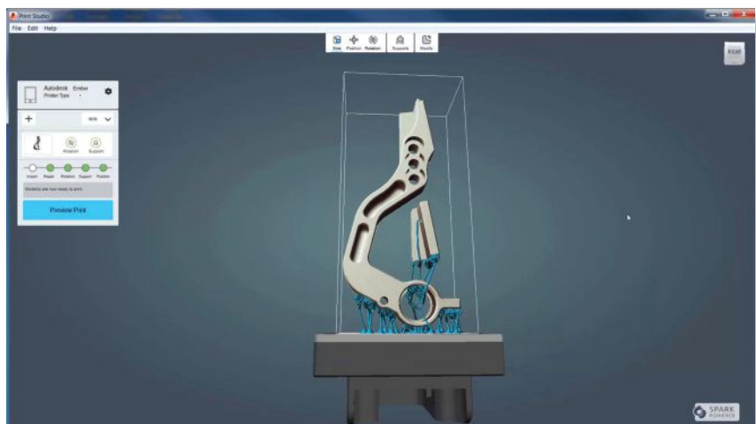
Autodesk Inventor 2016 comes with Print Studio, which generates the necessary support structures for 3D printing projects. Image courtesy of Autodesk.
